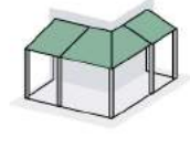
Circumferential pent roof
