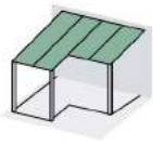
Pent roof with roof guttering offset
